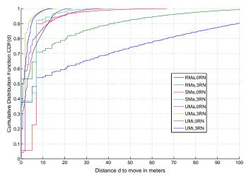
Fig. 4. CDF of the movement distance d for all IMT scenarios. 0 and 3 in the scenario name parameter mean the number of relay nodes in the cell.
